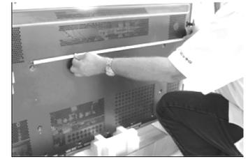
Prior to adjustment, loosen Slider Retaining Screws.
