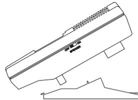
2. Insert the hooks into the slots and gently push the CID-932 down on the bracket to snap the bracket onto the CID-932.
