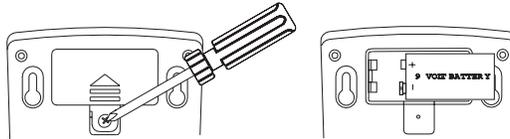
**Note:** The screw is packed separately. Insert the screw into the battery compartment cover when you first install the battery.
