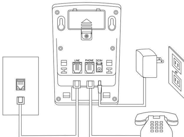
1. Unplug the telephone line cord from your telephone and plug it into the CID-932's **PHONE** jack.
