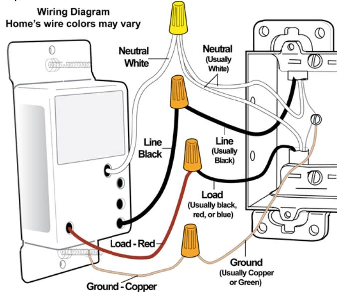
**Note:** the neutral wire will not normally be connected to the switch you are replacing. If there is no neutral wire in the box, consult an electrician or call the INSTEON Support line at 1-800-762-7845.
