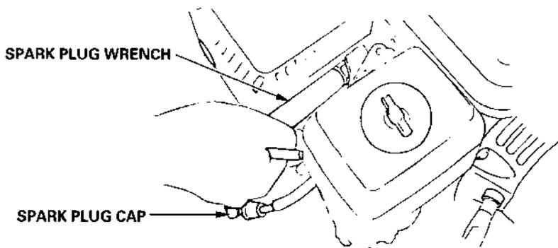
3. Inspect the spark plug. Replace it if the electrodes are worn, or if the insulator is cracked or chipped. Clean the spark plug with a wire brush if you are going to reuse it.
