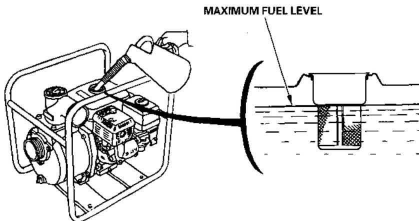
Refuel in a well-ventilated area before starting the engine. If the engine has been running, allow it to cool. Refuel carefully to avoid spilling fuel. Do not fill the fuel tank above the fuel strainer shoulder. After refueling, tighten the fuel tank cap securely.
