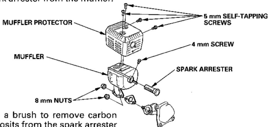
4. Use a brush to remove carbon deposits from the spark arrester screen. Be careful to avoid damaging the screen.
