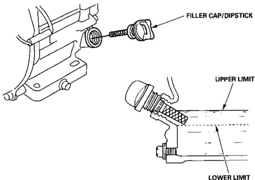
The Oil Alert® system will automatically stop the engine before the oil level falls below safe limits. However, to avoid the inconvenience of an unexpected shutdown, check the oil level regularly.
