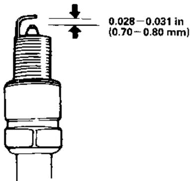
5. Install the spark plug carefully, by hand, to avoid cross-threading.
