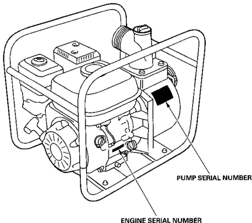
Record the pump serial number and the engine serial number in the space below. You will need these serial numbers when ordering parts, and when making technical or warranty inquiries (see page 60).
