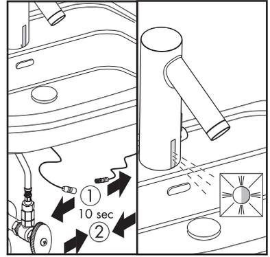
When the LED stays on, cover the sensor window with your hand or with a white card for 20 - 40 seconds to reset the electronics\*.
