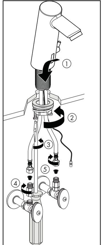
Tighten the hoses with two wrenches, as shown, to prevent the hoses from twisting.
