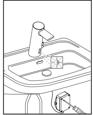
Remove the old battery (1). Install the new battery (2).
