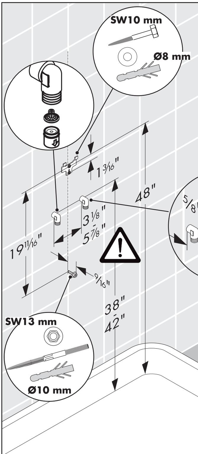
**!** Before drilling the bottom holes pay attention if hot and/or cold water supply pipes cross this area. In this case, only drill on the side without any supply pipes.
