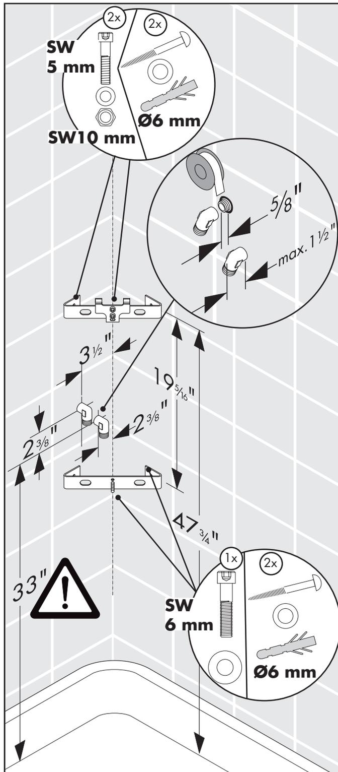
**!** Before drilling the bottom holes pay attention if hot and/or cold water supply pipes cross this area. In this case, only drill on the side without any supply pipes.
