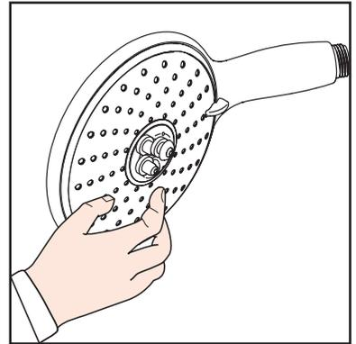
Remove scale deposits on the spray face by using a commercial limescale remover such as Lime-Away<sup>TM</sup> or CLR<sup>TM</sup>. Follow the label instructions carefully. Soak only the spray face.
