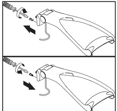
Attach the Allrounder to the mounting plate. Tighten the set screw.
