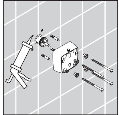
Remove the long bottom mounting screw on the All-rounder. Replace with the shorter screw included with the adapter.
