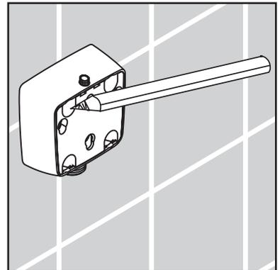
Drill the holes with a 6 mm bit. Use extreme caution - do not drill into the water line.
