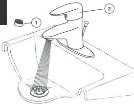
Remove aerator (1) and turn faucet handle (2) all the way on. Turn on hot and cold water supplies (3) and flush water lines for one minute.
