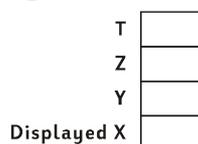
(For this reason, they are generally referred to as the “stack registers” or collectively as “the stack.”) The stack registers are designated X, Y, Z, and T. Unless the calculator is in Program mode, the number shown in the display is the number in the X-register (modified according to the current display format).
