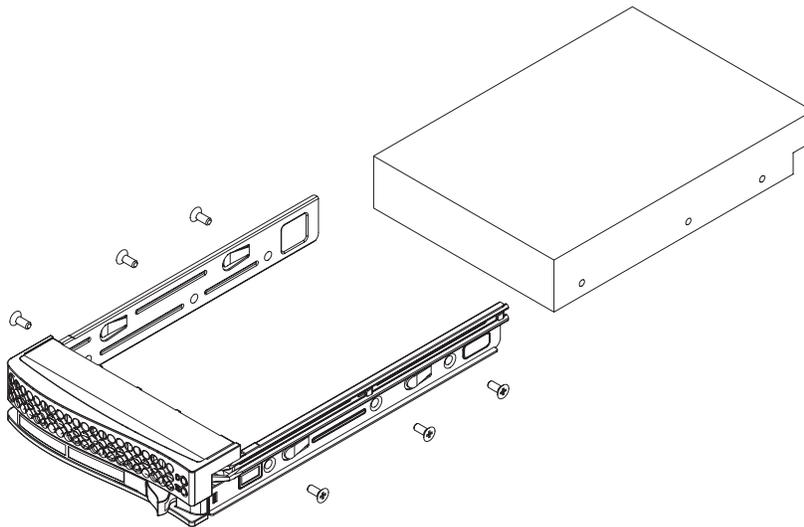
Figure 6-4. Mounting a SATA/SCSI Drive in a Carrier
