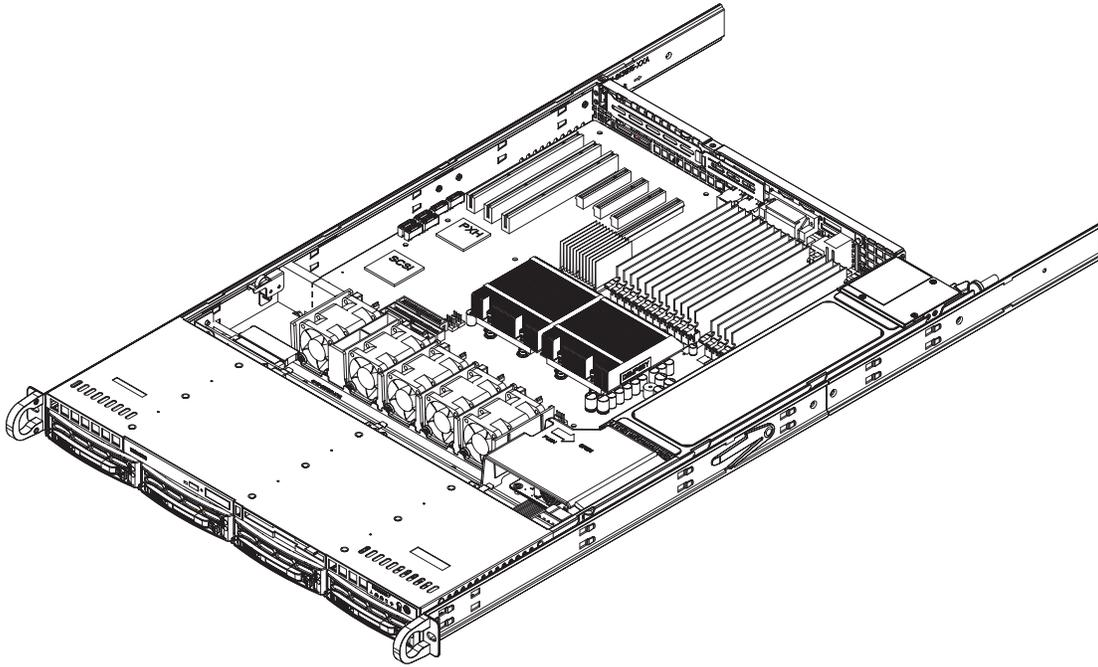
**Figure 2-5. Accessing the Inside of the System
