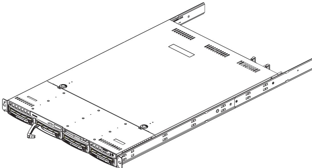
Figure 6-5. Removing a SATA/SCSI Drive from the Server
