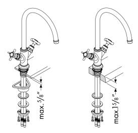
Attach the supply lines to the stops with 3/8" compression fittings (not included).
