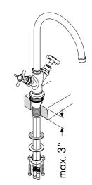
Place the faucet and sealing ring on top of the mounting surface.
