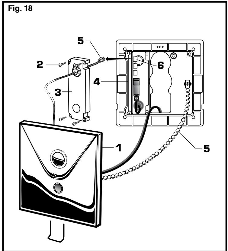
9. Replace the FRONT PANEL (1). See Step 9 for instructions on installing front panel.
