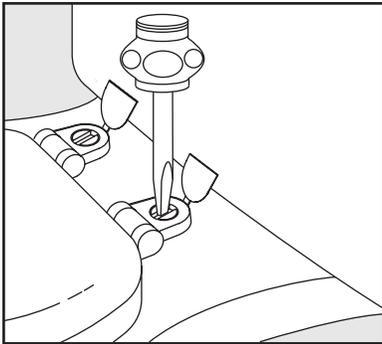
Use a screwdriver to tighten bolt.
