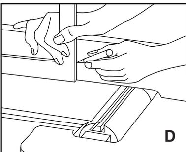
3. Remove Jointer Pal and place a steel square over this mark and scribe another heavy vertical line on the fence (**see sketch D at left**). You now have two heavy vertical lines on the fence, about 4" apart. With the square in the same location, flip it down so it rests flat on the outfeed table and at a right angle with the fence. Scribe a 90° line across the outfeed table corresponding exactly with the rear vertical line on the fence.
