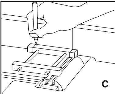
1. Leaving the cutterhead at TDC, mark a corresponding spot on the fence using a steel square and black felt-tip marker. With the steel square in the same position, scribe (scratch) a heavy vertical line on the fence directly in line with the high point of rotation of the topmost knife. Use a scribe or any sharp tool that is harder than your jointer’s fence. **See sketch B at left.**
