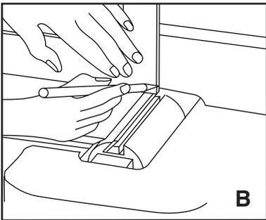
1. Locate the high point of the cutterhead rotation by placing a straightedge (wood or metal) on the outfeed table and extending it over the cutterhead. **See sketch A at left.**
