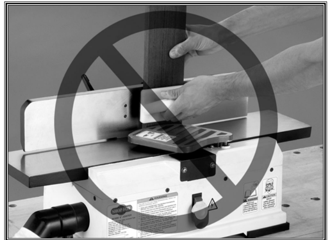
Figure 5. Never joint end grain!
