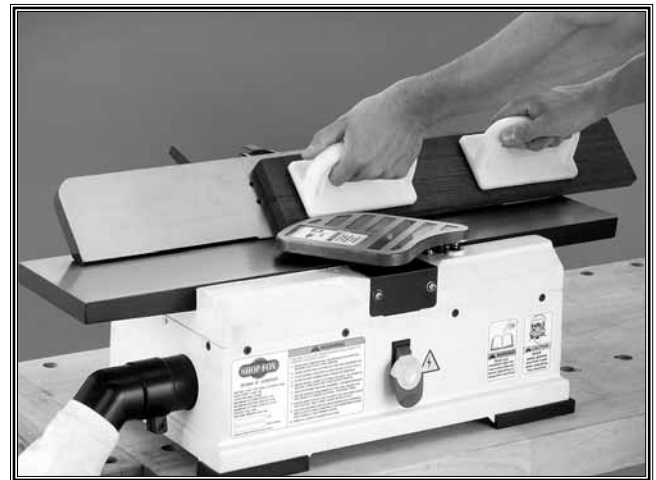
Figure 37. This is an example of a bevel cutting operation with the fence set at 45°.
