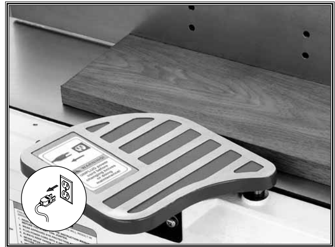
Figure 30. Blade guard in use.
