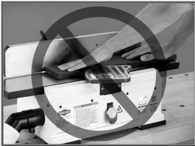
Figure 2. Never surface plane without push blocks!
