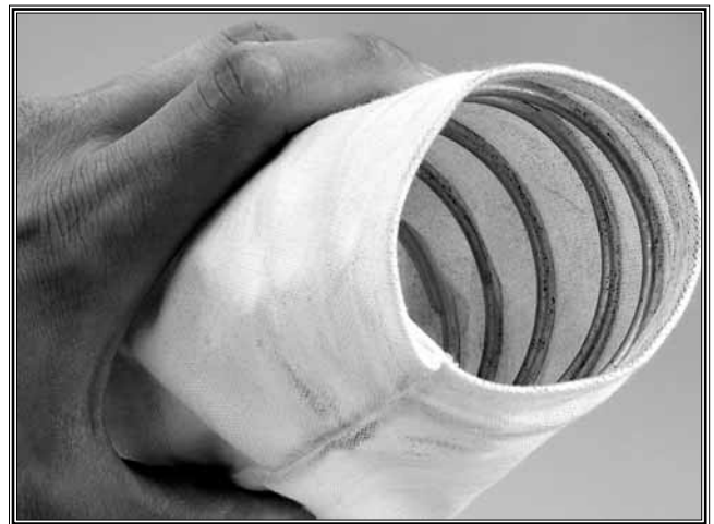
Figure 15. Correctly installed filter bag spring.
