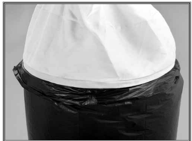
Figure 19. Filter bag secured to the trash bag.
