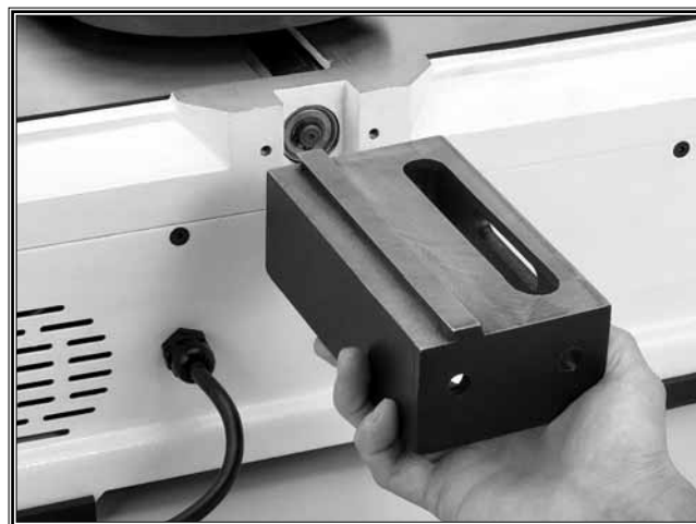
Figure 9. Aligning the fence support.
