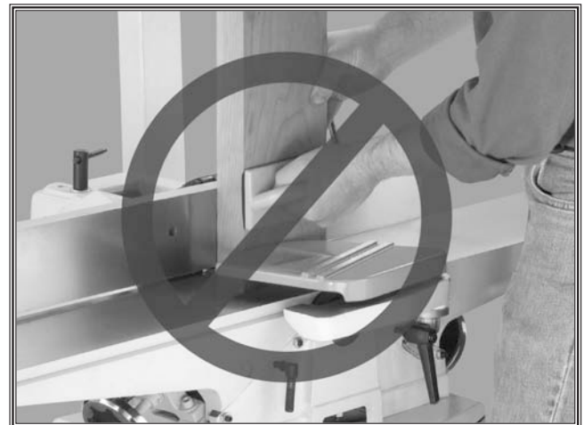
Figure 7. Never joint end grain!
