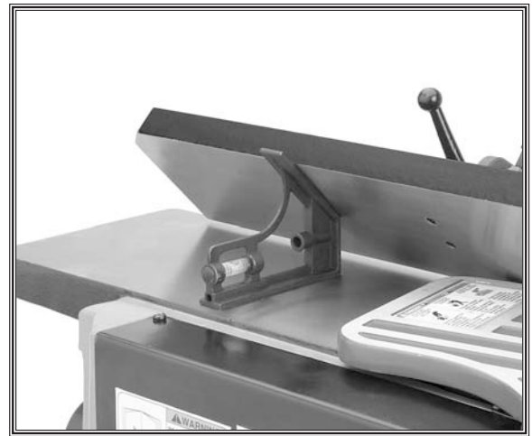
Figure 42. Checking the inward 45° stop.
