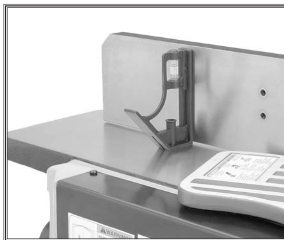
Figure 41. Checking the 90° stop.
