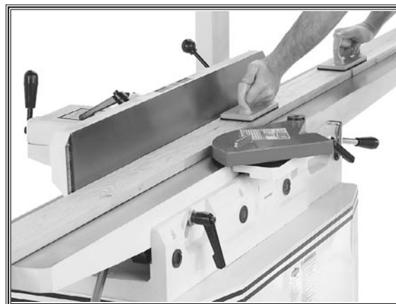
Figure 34. Typical surface planing operation.
