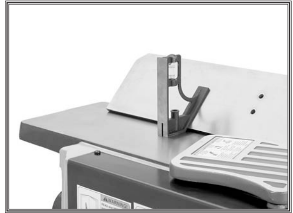
Figure 44. Checking the outward 45° stop.
