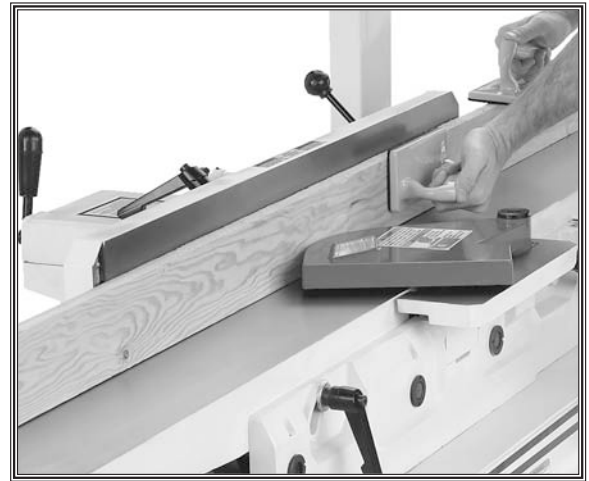
Figure 36. Typical edge jointing operation.
