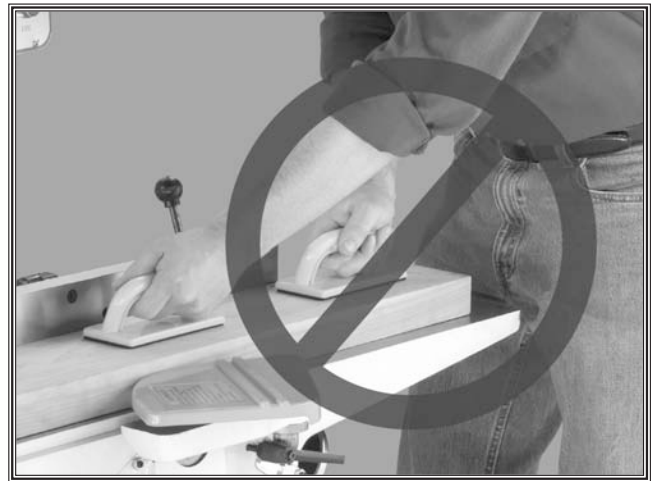
Figure 6. Never stand directly behind the workpiece!
