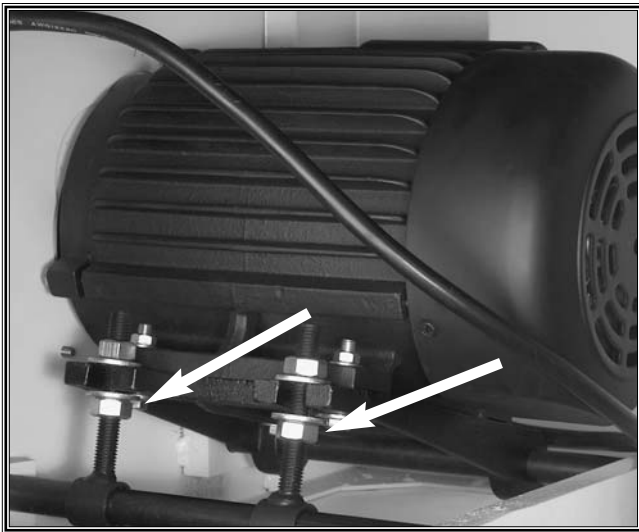
Figure 40. V-belt adjustment check nuts.
