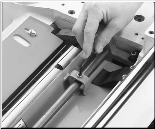
Figure 22. Chipbreaker adjustment controls.
