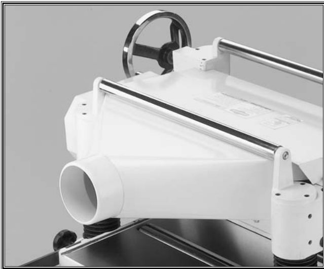
Figure 5. Dust hood attached to planer.
