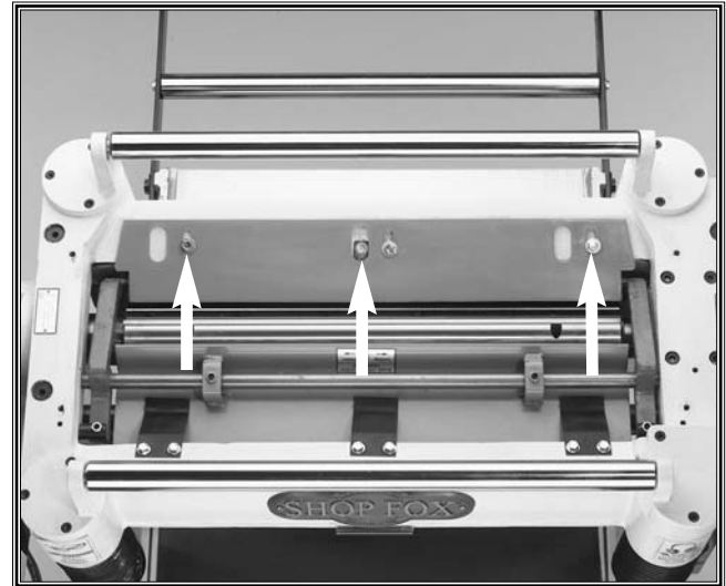
Figure 24. Chip deflector mounting bolts.
