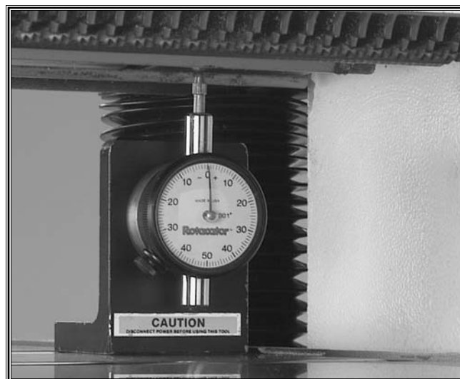
Figure 34. Measuring table-to-cutterhead with Rotacator® in upward position.
