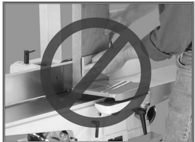
**Figure 5.** Never joint end grain!
