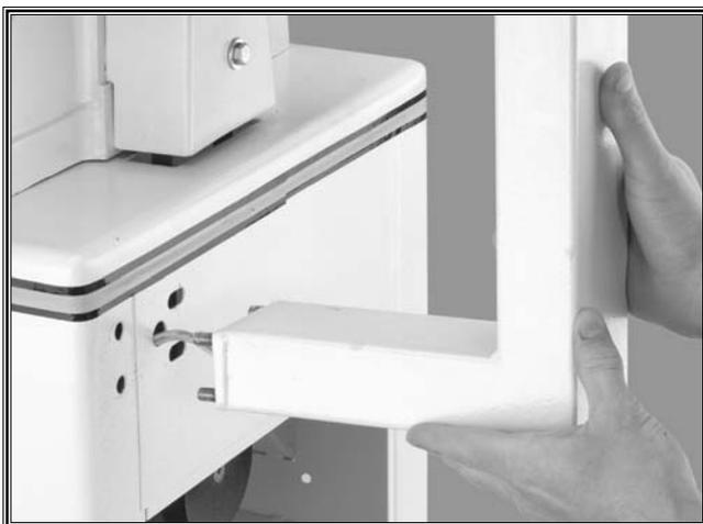
**Figure 20.** Mounting pedestal switch to stand.
