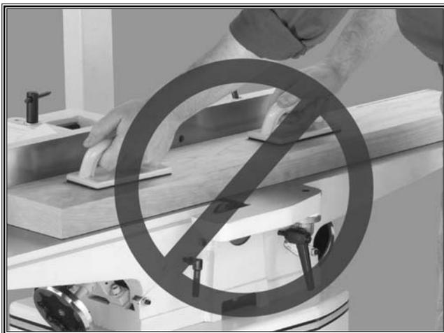
**Figure 4.** Never plane/edge-joint with the guard removed!
