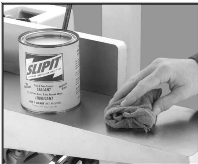
Figure 43. Applying lubricant to table surface.
