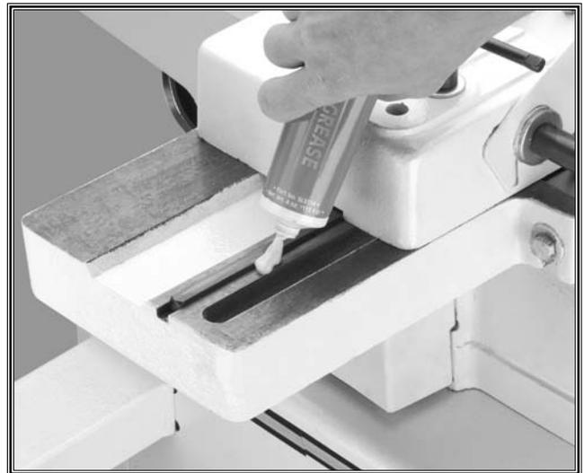
**Figure 45.** Greasing fence keyway.
