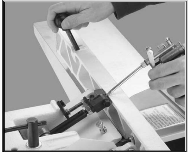
**Figure 44.** Lubricating fence pivot points.
