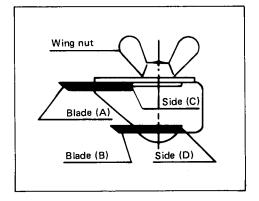
Immerse the dressing stone in water for 2 or 3 minutes before sharpening. Hold the holder so that the blades both contact the dressing stone for simultaneous sharpening at the same angle.
