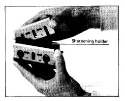
First, loosen the two wing nuts on the holder and insert the blades (A) and (B) so that they contact the sides (C) and (D). Then tighten the wing nuts.
