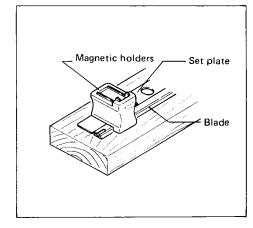
Lock the drum in the position whereby the blade installation bolts face upward. Place the set plate and blade on the drum so that the heads of the depth adjusting screws in the drum fit into the square holes in the set plate. Remove the magnetic holders while holding the set plate with your hand.
