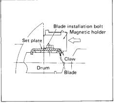
After tightening all the blade installation bolts lightly and evenly from the center to the outside, tighten them completely following the same sequence. Remove the magnetic holders from the set plate.
