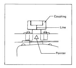
Align the two shafts of the jointer with the mating holes in the auto-planer. Push the jointer toward the auto-planer until the frame of the jointer contacts that of the auto-planer. Make sure the jointer is correctly installed on the auto-planer by viewing the contact portion through the notch. Tighten the knobs to secure the jointer. Re-install the fence and tighten the clamp screws to secure the fence.
