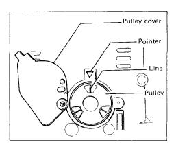
Loosen the clamp screws which secure the fence. Remove the fence. Align the line on the coupling with the pointer on the frame of the jointer.
