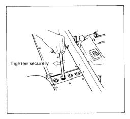
Then slightly retighten the adjusting screws by turning clockwise.
