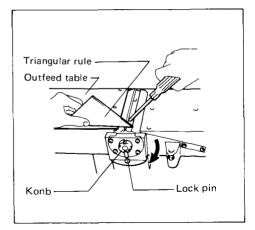
After carefully adjusting the blade protrusion, lock the drum in the position whereby the blade installation bolts face upward. Securely tighten the blade installation bolts evenly from the center of the outside
