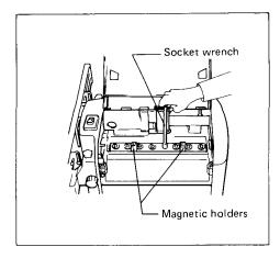
Install the other blade as described above. Rotate the drum slowly while pressing the lock plate to make sure there is nothing abnormal. Then close the chip cover and secure using the hex bolt.
