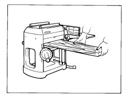
Two rollers are provided on top of the tool to enable quick, effotless return of the workpiece to the infeed table side. This is especially convenient with two operators.
