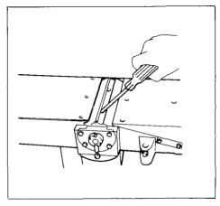
Install the other blade as described above. Re-install the safety cover in its original position and be sure that the safety cover works properly and briskly.
