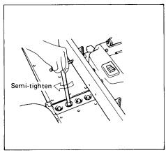
Lock the drum in the position whereby the blade edge faces upward. Place the triangular rule flat on the outfeed table. Turn the adjusting screws until the blade edge just contacts the triangular rule. After adjusting both adjusting screws, pull the lock pin to unlock the drum. Rotate the drum by turning the knob clockwise to make sure the blade protrusion is at exactly the same height all the way across. If not, adjust the adjusting screws again.
