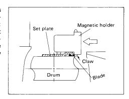
Grip the magnetic holders and raise them to remove the set plate and blade from the drum. Pull the lock pin and rotate the drum by turning the knob 180° to lock the drum. Remove the other blade as described above.
