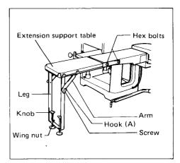
When moving the tool, fold the extension support table as follows.
