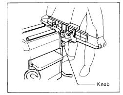
When the jointer is removed, the pulley cover will close automatically. If you lock the pulley cover in the open position for some reason, be sure to close it by pushing the release button before operating the auto-planer. Never operate the auto-planer with the pulley cover locked in the open position.
