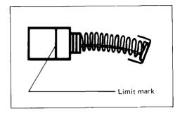
Open the chip cover and remove the brush holder caps using a screwdriver. Take out the worn carbon brushes, insert the new ones and secure the brush holder caps.
