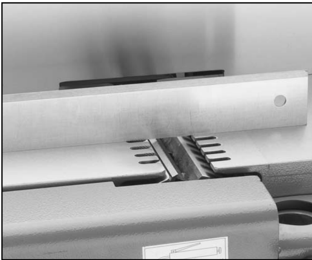
Figure 13. Setting the depth of cut scale.
