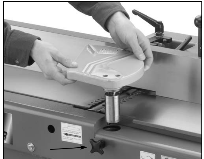
Figure 6a. Attaching cutterhead guard.
