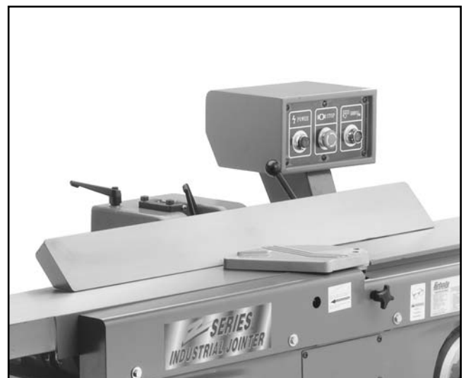
Figure 20. Fence position for bevel jointing.
