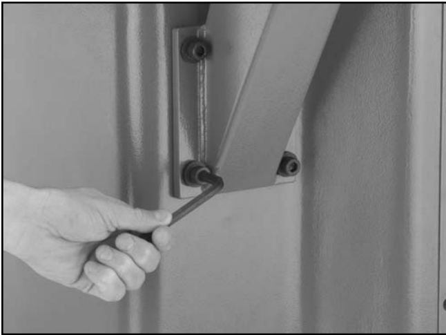
Figure 7A. Mounting the pedestal switch.
