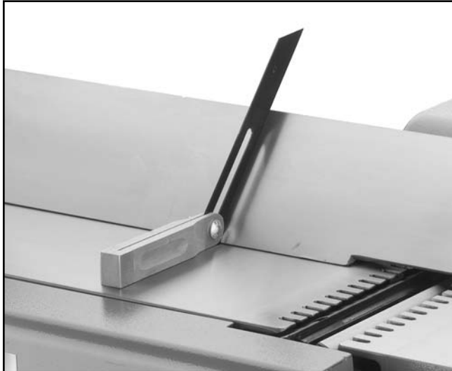
Figure 16. Using a 45° gauge to align fence.
