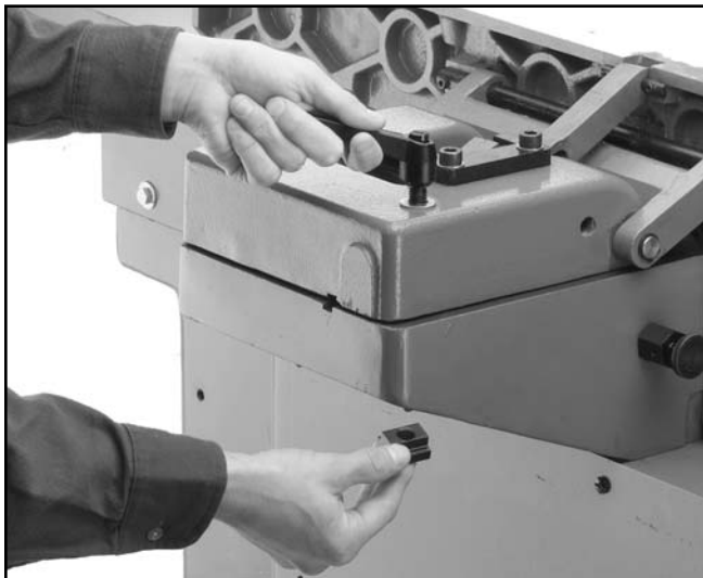
Figure 5. Fence base lock knob attachment.
