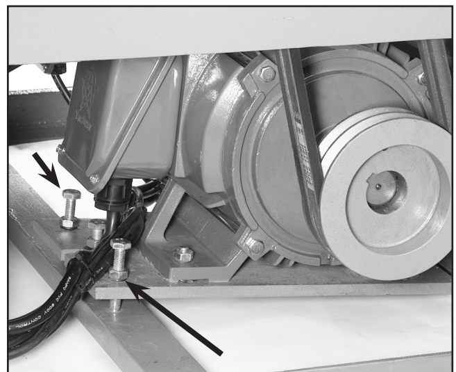
Figure 23. Motor mount adjustment bolts.
