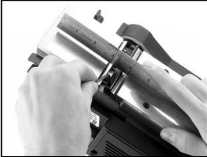
**Figure 10.** Setting cutter height.
