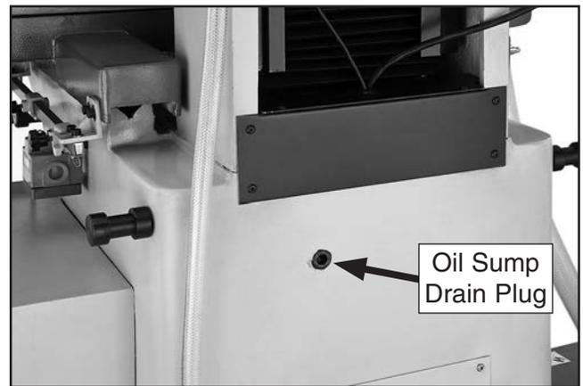
**Figure 46.** Location of oil sump drain plug.
