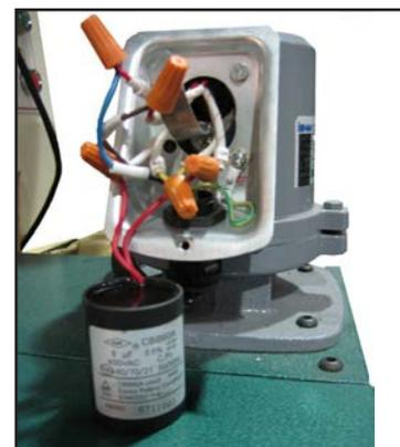
Figure 56. Coolant motor wiring (220V).
