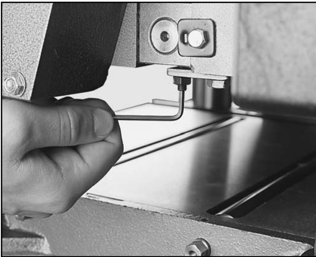
Figure 20. Feed roller height adjustment.
