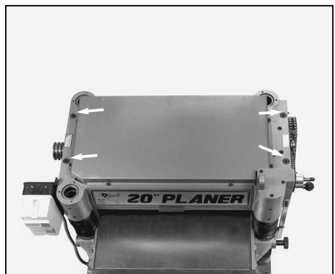
Figure 41. Feed roller lubrication points.
