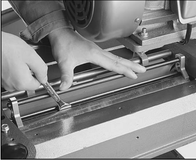
Figure 16. Tightening knives in cutterhead.
