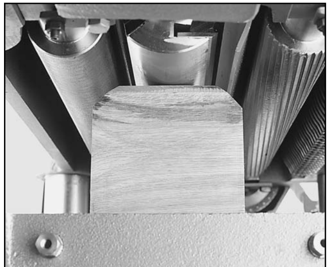
Figure 12. Guide block indicates parallelism.
