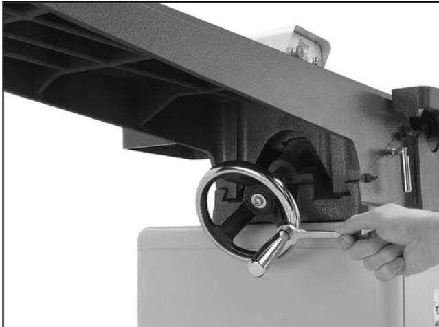
**Figure 16.** Securing the handwheel handle.
