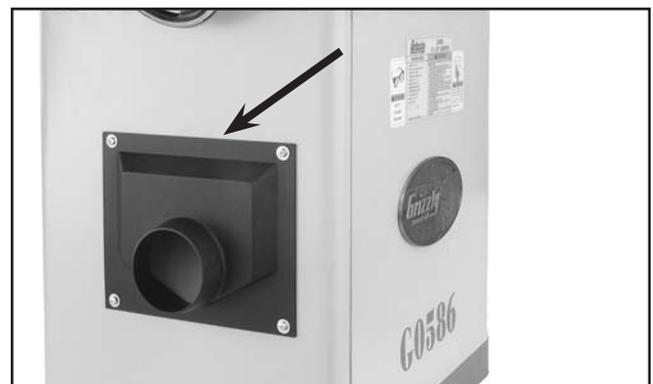
**Figure 15.** Correctly installed dust port.
