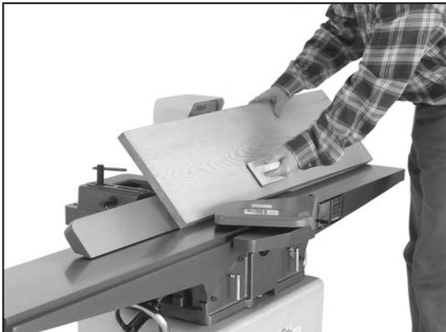
**Figure 26.** Typical bevel cutting operation.
