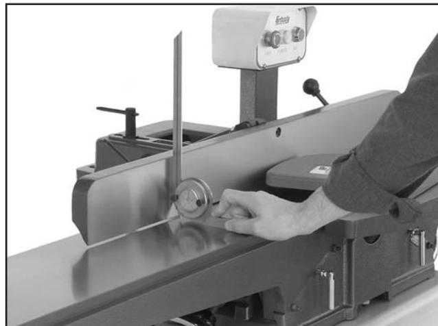
**Figure 49.** Adjusting fence to 90°.
