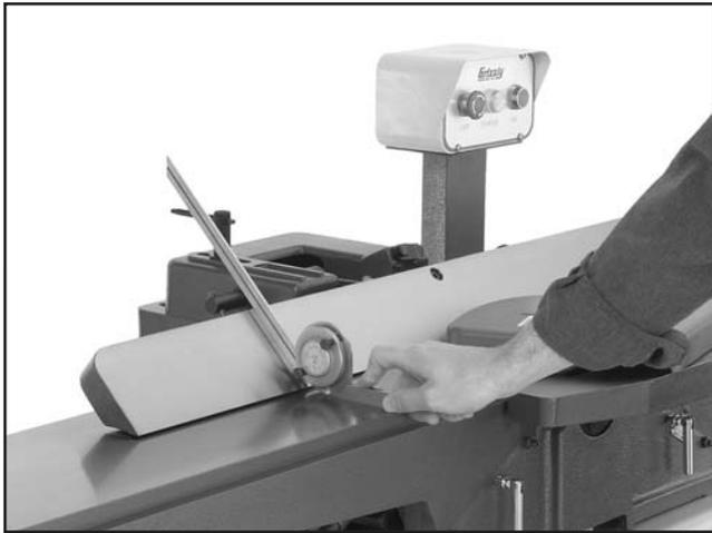
**Figure 51.** Adjusting fence 45° outward.
