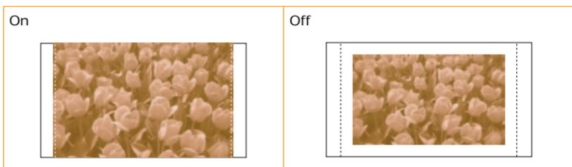
Selecting borderless 'off.' shrinks the image slightly to allow an empty border around the image.
