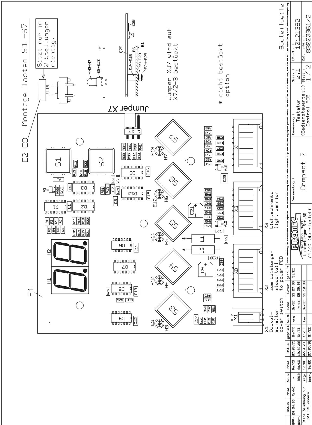
Important: For machine type COMPACT 2 Jumper no. X7 should be placed in pos. 2-3.
