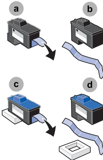
**Warning:** Do not touch the gold contact areas on the back and bottom of the cartridges.
