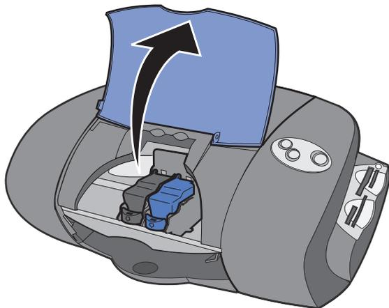
If the cartridge carrier does not move to the center position, see page 16 for help.
