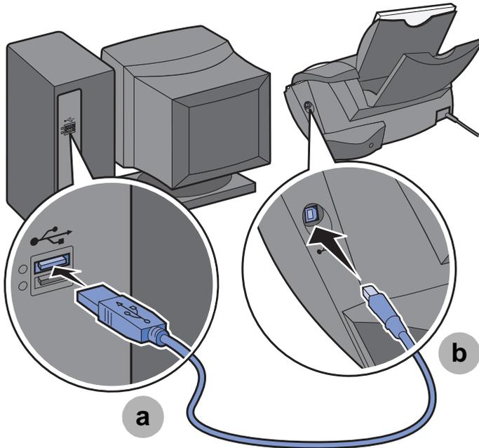
**Note:** The location and orientation of the USB port on your computer may be different from the one shown. Check for this symbol:
