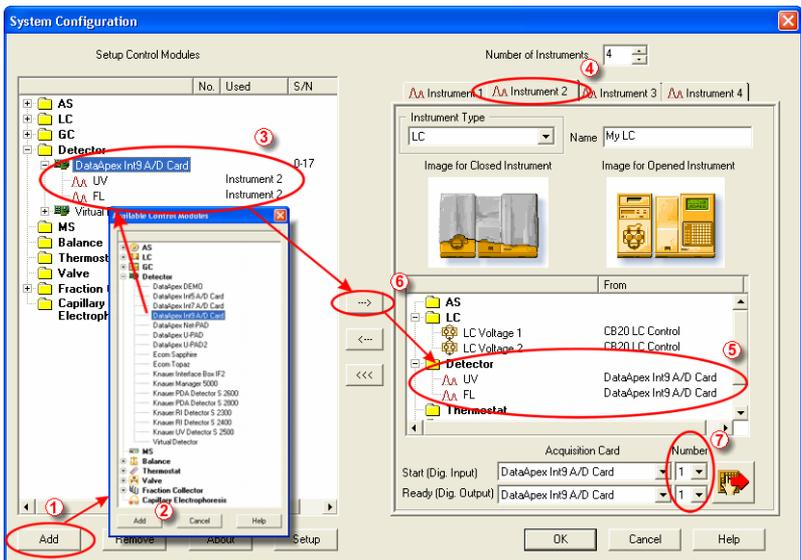
**Fig. 4. System Configuration**
