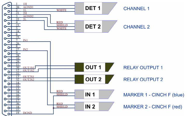
**Fig. 14. Standard INT7-compatible cable for two detectors**
