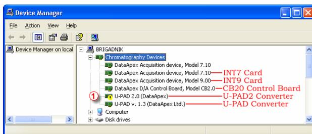
If the "DataApex Acquisition device, Model 9.xx" item is missing, Windows has automatically installed an incorrect driver.
