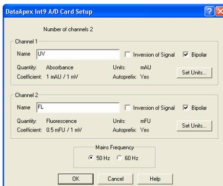
**Fig. 3. INT9 A/D Card Setup**
