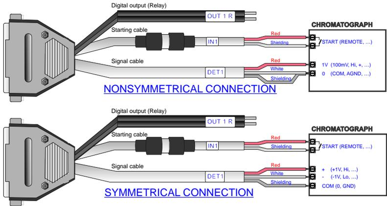
**Fig. 2. Connecting Clarity to chromatograph**
