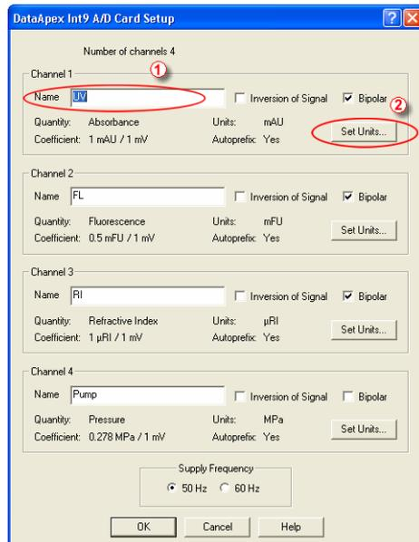
**Fig. 8. INT9 A/D Card Setup**
