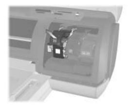
5 If you are replacing a print cartridge, slide the old print cartridge out and store, recycle, or discard it.
