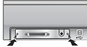
tighten the two mounting screws
