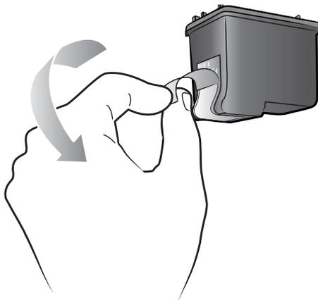
**Caution!** Do not touch the ink nozzles or the copper contacts on the print cartridge. Touching these parts may cause the print cartridge to fail.
