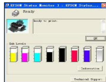
If the indicator light flashing when printing, it tells that you need to reset the chip to full status. Please turn off your printer for about 1 minutes and switch it back on. Ink meter bar shall show full ink. You can start printing as usual.
