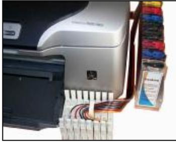
Put the CISS on the left side of the printer. In the meantime place all the tubes at correct position.
