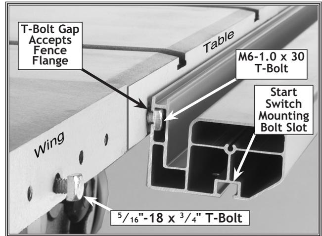
**Figure 8.** Front rail being slid onto T-bolts.
