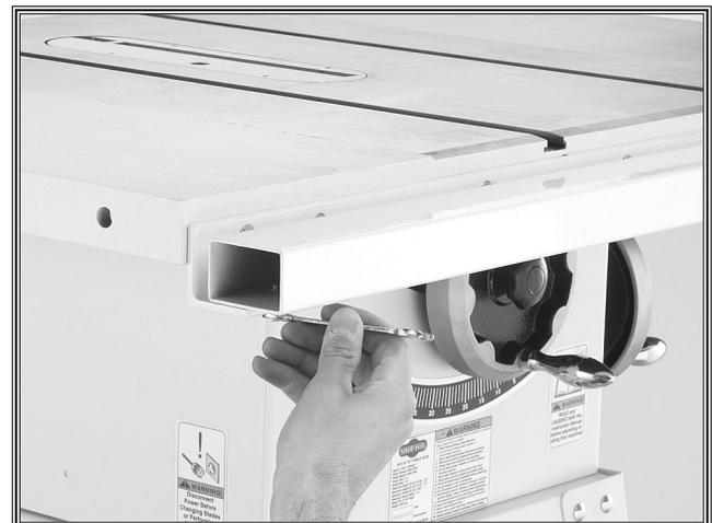
Figure 4. Installing fence tubing.
