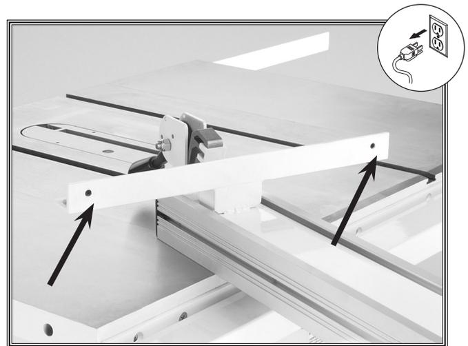
Figure 13. Fence adjustment setscrews.
