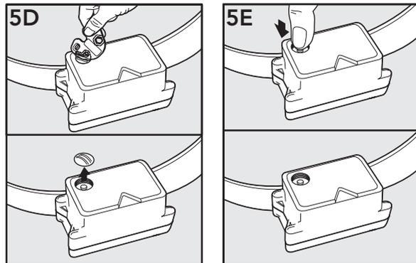
The Static Correction levels increase in strength from 1 to 5. Pushing the Correction Level Button while the Receiver Collar is on level 5 will cause the Receiver Collar to revert to Level 1. Refer to the Function and Response Table to choose the Static Correction level that best fits your pet.
