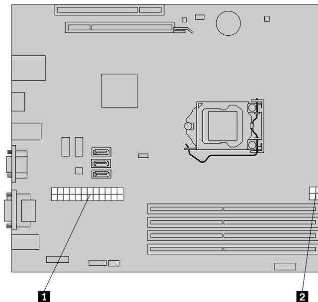
Figure 22. Power connectors on the system board
