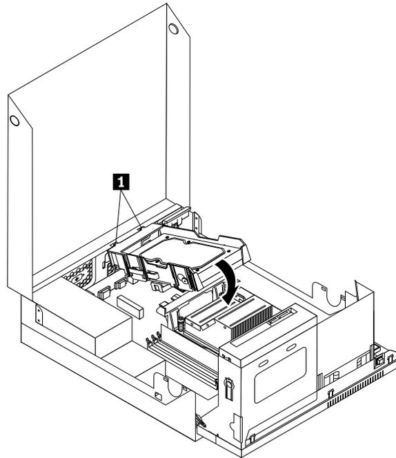
Figure 17. Installing the hard disk drive
