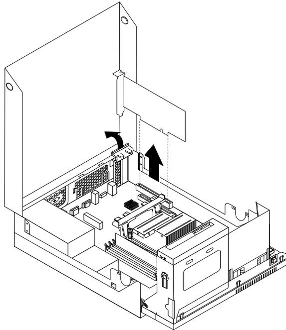
Figure 11. Removing a PCI card
