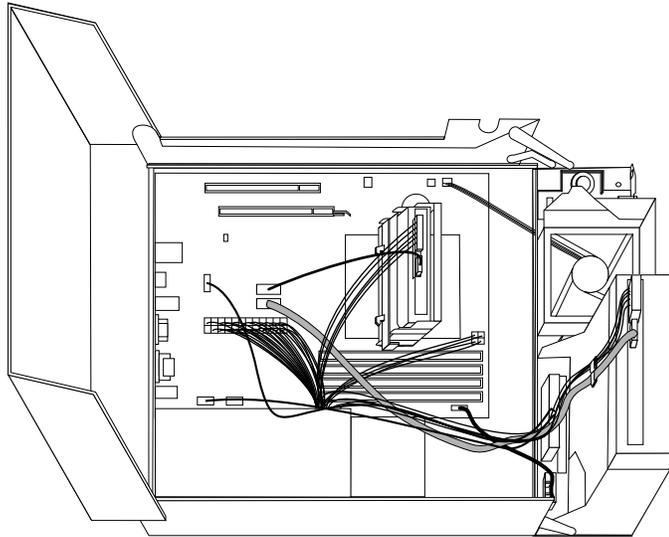
Figure 32. Cable routing
