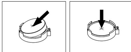
Figure 14. Installing a new battery
