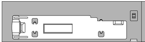
*Figure 19. Installing the optical drive retainer*
