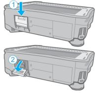
Connect the USB device to the USB port.
