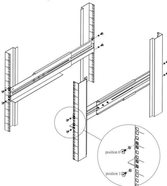
Place the Step-Down Transformer on a flat stable surface with the front of the unit facing toward you. Secure the Step-Down Transformer to your rack with four M5X12L screws at the front of the rack. The 2U Step-Down Transformer takes up position 2 through position 5. The 3U Step-Down Transformer takes up position 2 through position 8.
