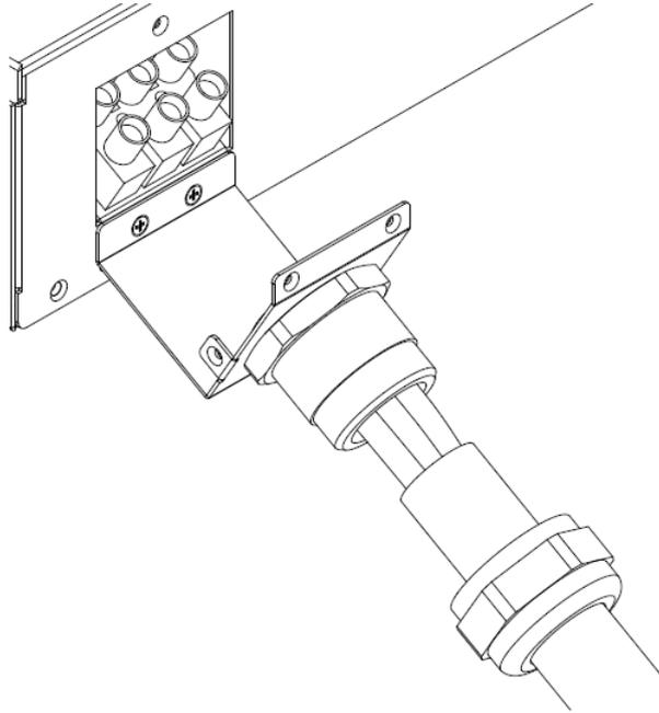
Connect the three wires to the input terminal block.
