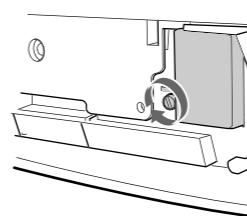
Match the projection of the right side of the lamp cover with the hole of the unit, and replace the lamp cover as it was.
