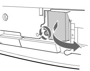
**6** Loosen the two screws that secure the lamp, then pull out the lamp.
