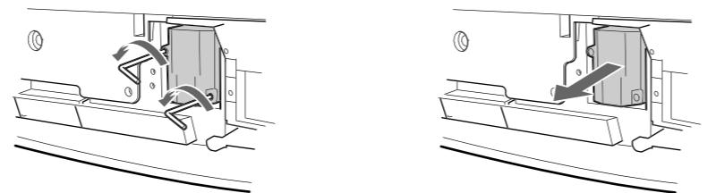
Loosen the two screws with the supplied hex key.
