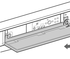
Push and release the center in the upper of the control panel cover to open it.
