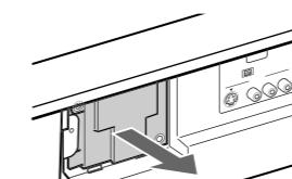
Loosen the two screws as shown in the illustration using the supplied hex key.
