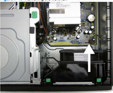
To install the front fan, reverse the removal procedure. Be sure to orient the air flow into the unit.
