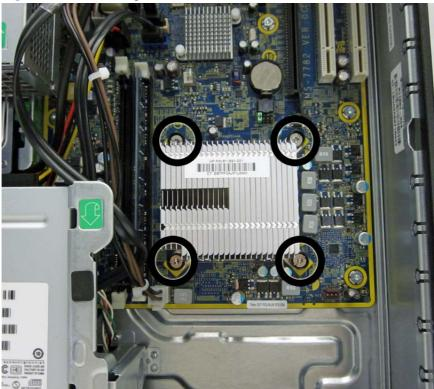
Lift the heat sink from atop the processor and set it on its side to keep from contaminating the work area with thermal grease.
