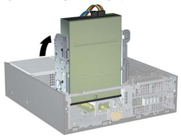
**4.** Rotate the power supply to its upright position. The hard drive is located beneath the power supply.
