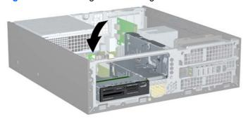
5. Slide the drive back until it stops, then lift it up and out of the drive cage.
