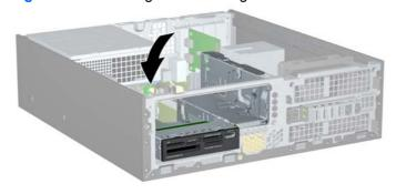
If installing a media card reader, connect the USB cable from the media card reader to the USB connector on the system board labeled MEDIA1.
