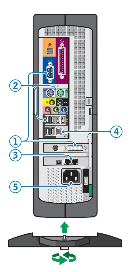
See your *Owner's Manual* for instructions on attaching the stand. The screw is attached to the bottom of the stand.
