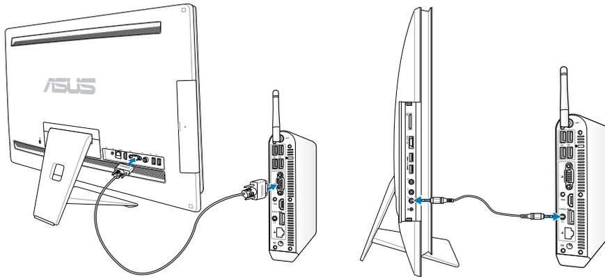
5. An **Input Select** OSD menu appears when you connect the HDMI or VGA cable to the rear HDMI-input or Display-input port. Use the **Volume Increase** (▲/+) / **Decrease** (▼/-) buttons to select **HDMI with Device Share** or **VGA with Device Share** press the **MENU** button to activate the option.
