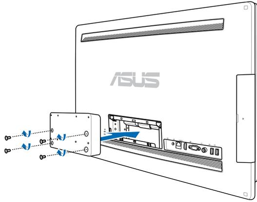
5. Secure the wall mount pad to the adapter with the eight screws (M3 x 8L) that came with the kit, noting the correct orientation.
