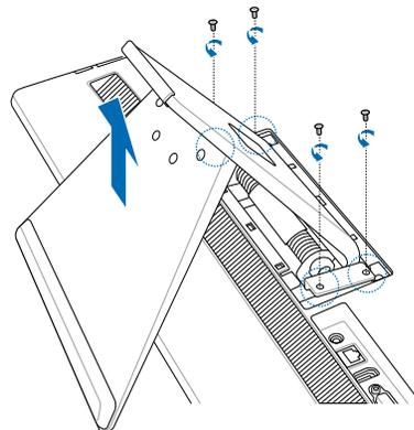
4. Align the wall mount adapter to the holes at the back of the All-in-one PC and secure it with the four screws you removed in step 3
