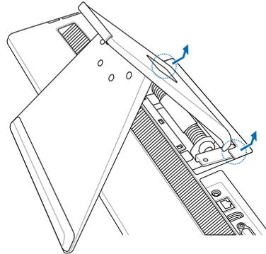
3. Remove the four screws on the stand and save for future reinstallation. Take out the stand and put it aside.
