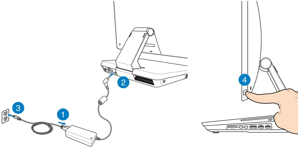
**WARNING!** DO NOT connect the AC power cord to an AC outlet prior to connecting the DC plug to the system. Doing so may damage the AC-DC adapter.
