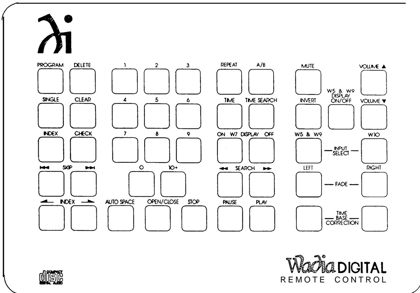
**MUTE:** Places the Wadia 9 Decoding Computer in / out of mute. Mute on the Wadia 9 Decoding Computer is at absolute zero, or at no volume. Pressing the MUTE button again, or either of the VOLUME buttons, will take the unit out of MUTE.
