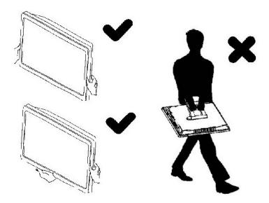
[Attention] Hold firmly when carry the computer, do not grasp the support frame directly.
