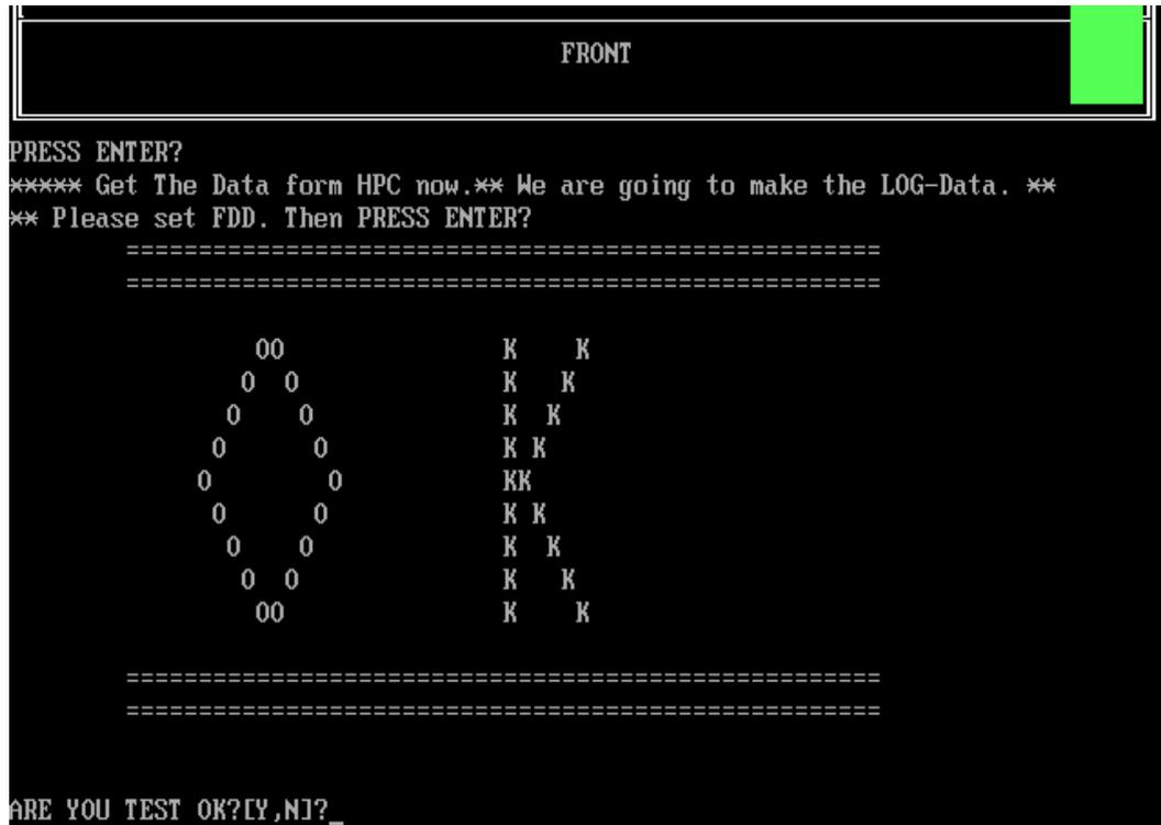
If the picture shows as below, it means the 3D G-sensor function is NG
