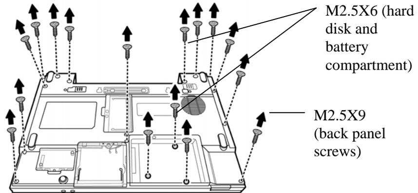
Figure 4-43 Removing the top cover (back panel screws)
