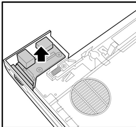
*Figure 4-69 Removing the VGA module*
