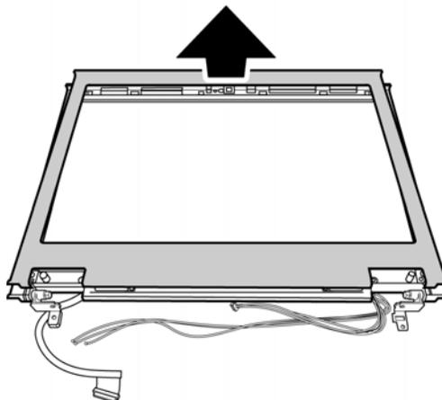
Figure 4-71 Removing the display mask
