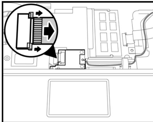
Figure 4-22 Disconnecting the FFC cable
