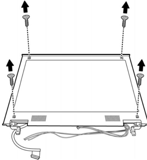
Figure 4-70 Removing the display mask screws
