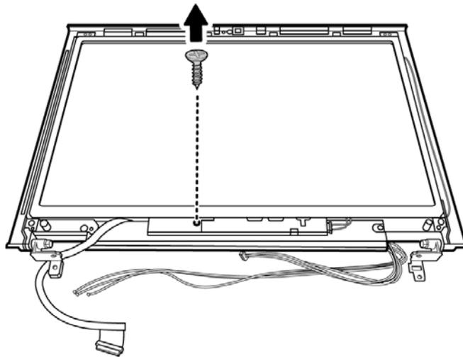
Figure 4-74 Removing the screws
