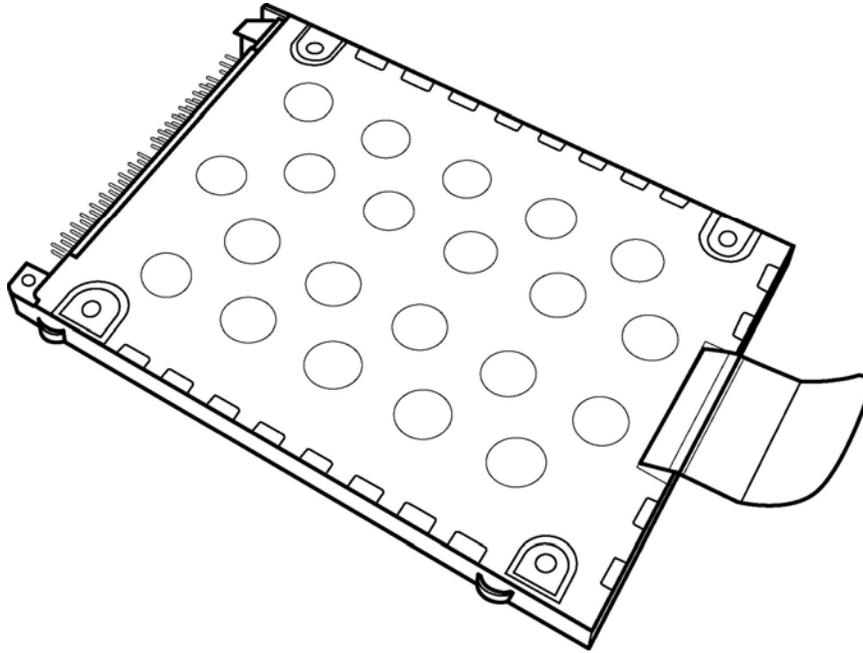
Figure 1-1 2.5-inch HDD
