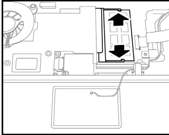
Figure 4-54 Releasing the memory module
