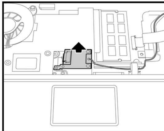
Figure 4-24 Removing the Bluetooth module
