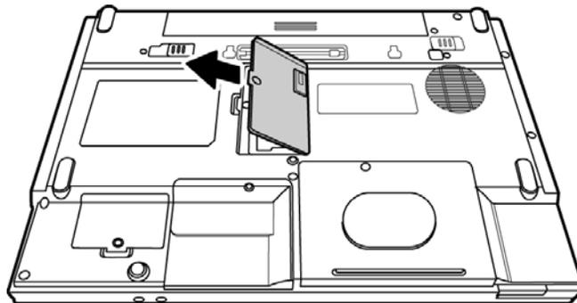
Figure 4-10 Removing the expansion memory module cover
