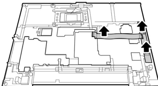
Figure 4-49 Removing the direct play button module
