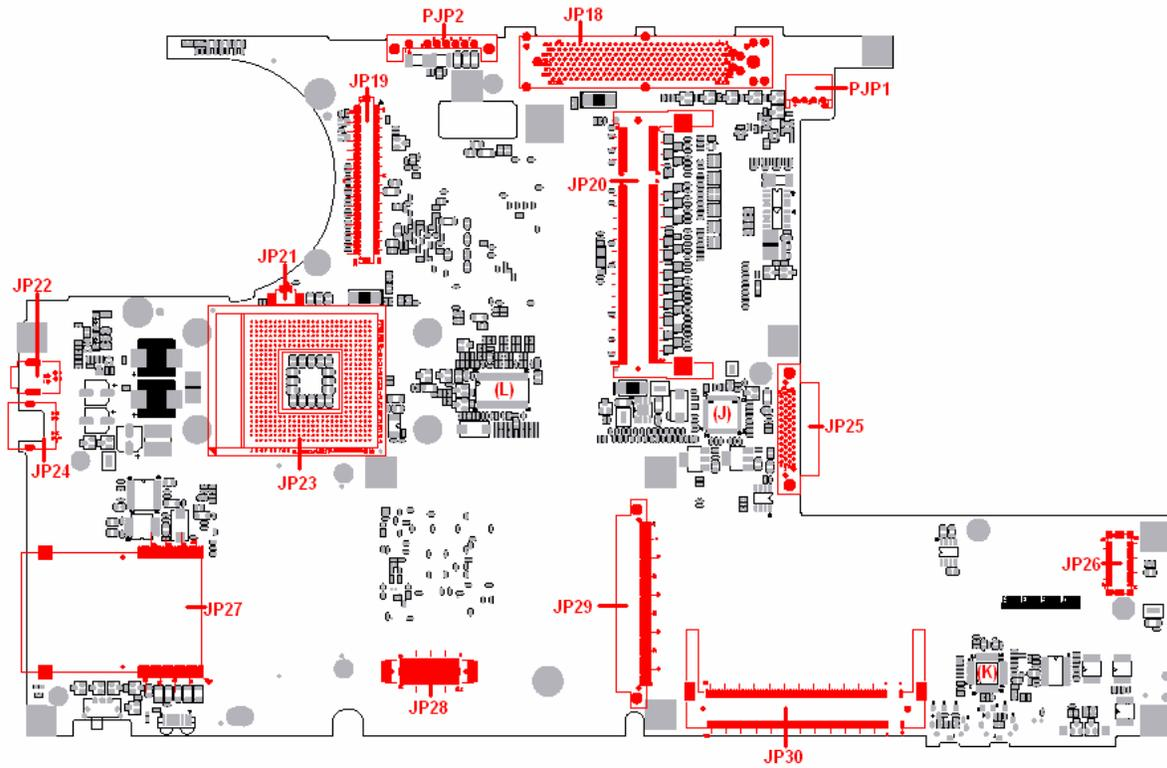
Figure B-2 System board (FRDSY\*) layout (Button)
