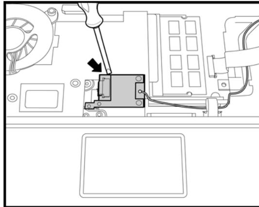
Figure 4-23 Lifting the Bluetooth module
