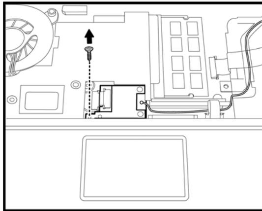
Figure 4-21 Removing the Bluetooth module screw
