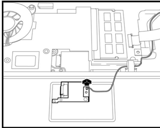
Figure 4-25 Disconnecting the Bluetooth connector
