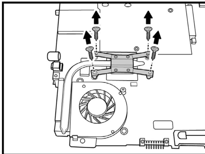
*Figure 4-60 Removing the heat sink screws*
