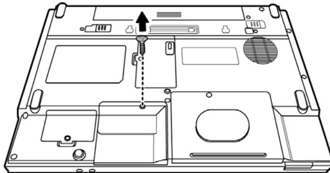
Figure 4-28 Removing the wireless LAN unit screw
