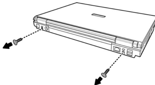
Figure 4-38 Disconnecting the rear screws
