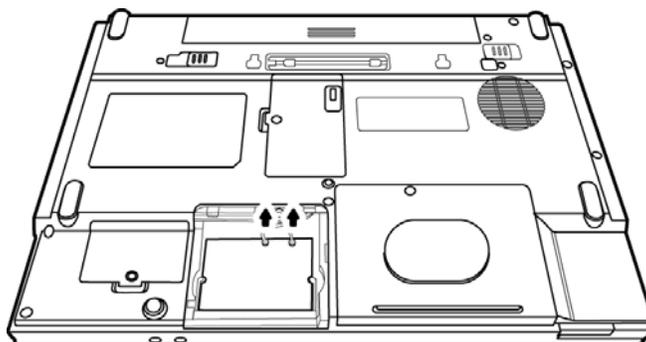
*Figure 4-30 Removing the wireless LAN antenna connectors*
