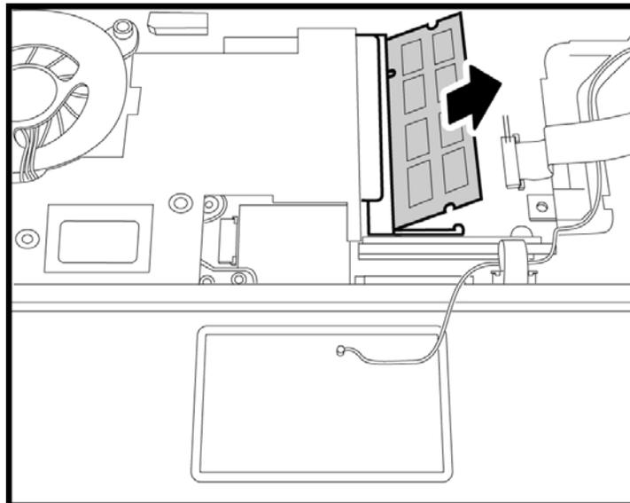
Figure 4-55 Removing the memory module
