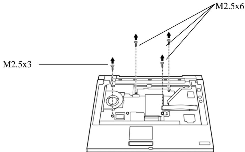
Figure 4-41 Removing the top cover (front panel screws)
