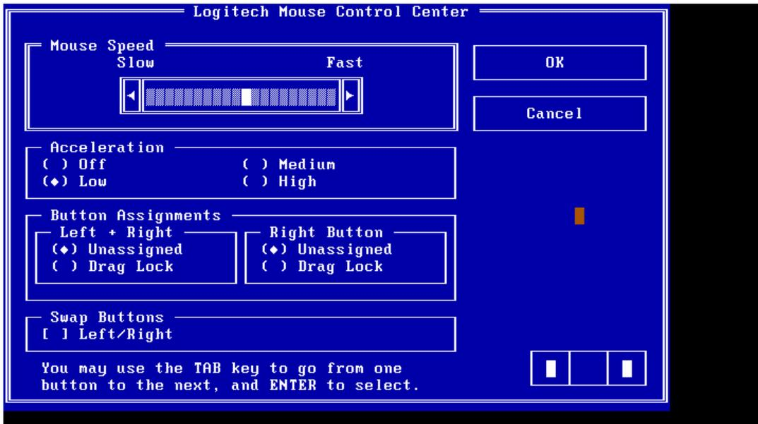
After checking T/Pad buttons and cursor's function, use "Tab" key or use T/Pad cursor to click the "OK" column will end this test.
