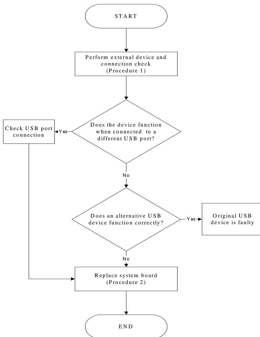
Figure 2-5 External USB device troubleshooting process
