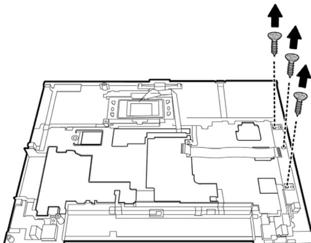
Figure 4-48 Removing the direct play button module screws
