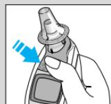
IRT 4520: Clear the display by pushing the «I/O» button once.
