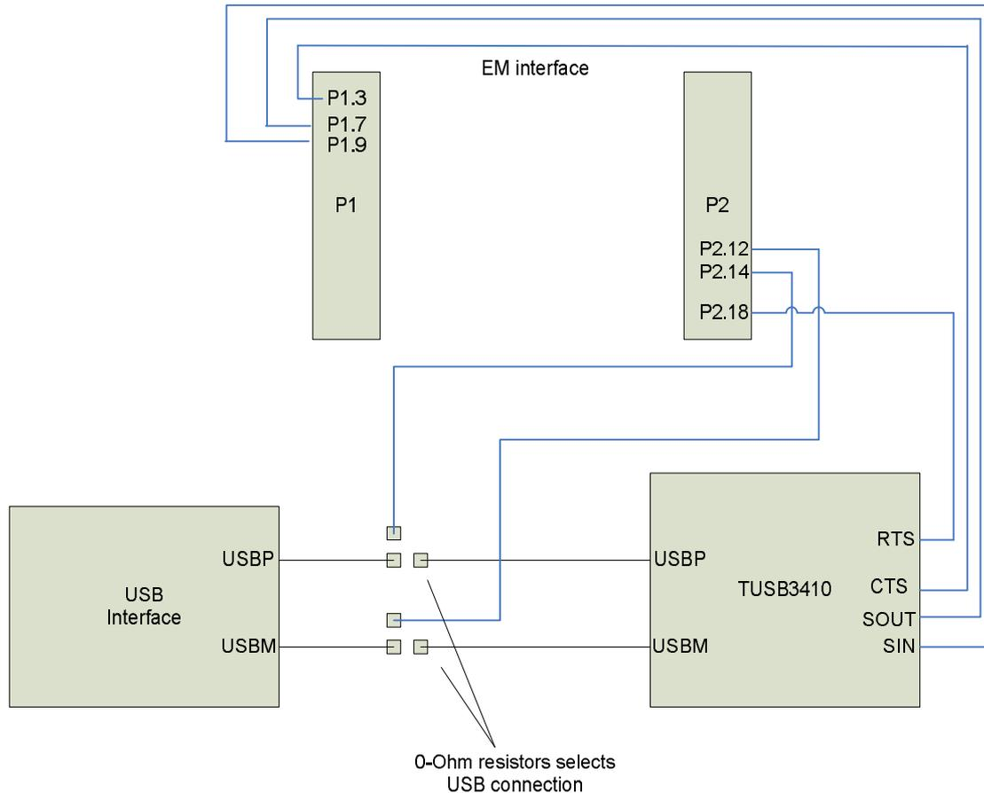
**Figure 11: USB interface selection with 0-ohm resistor**
