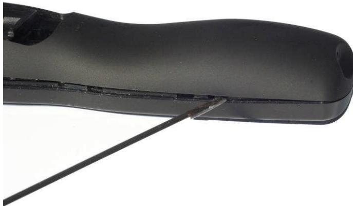
**Figure 15: Opening the remote control, step two**
