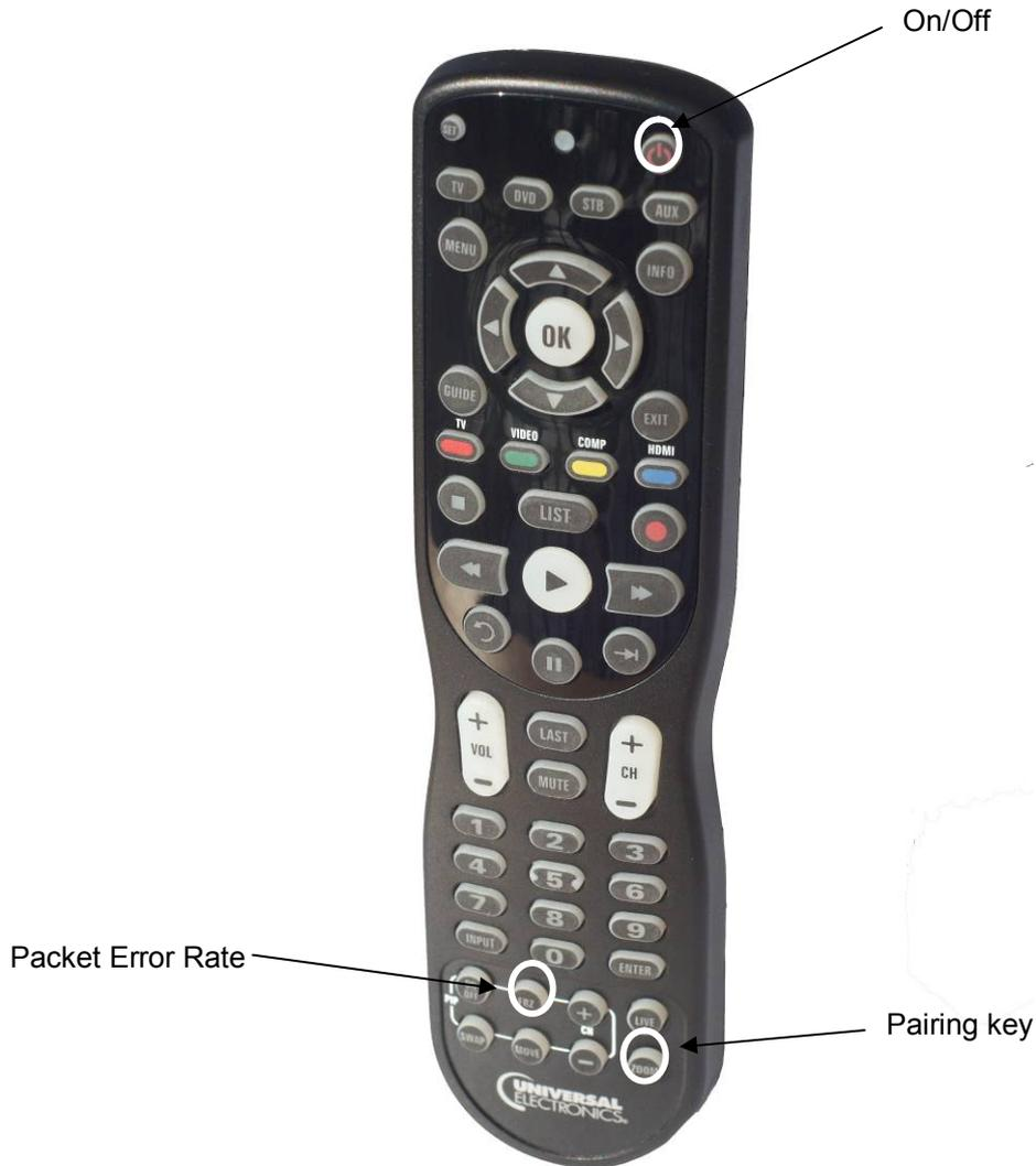
**Figure 1: Remote Control Key layout**
