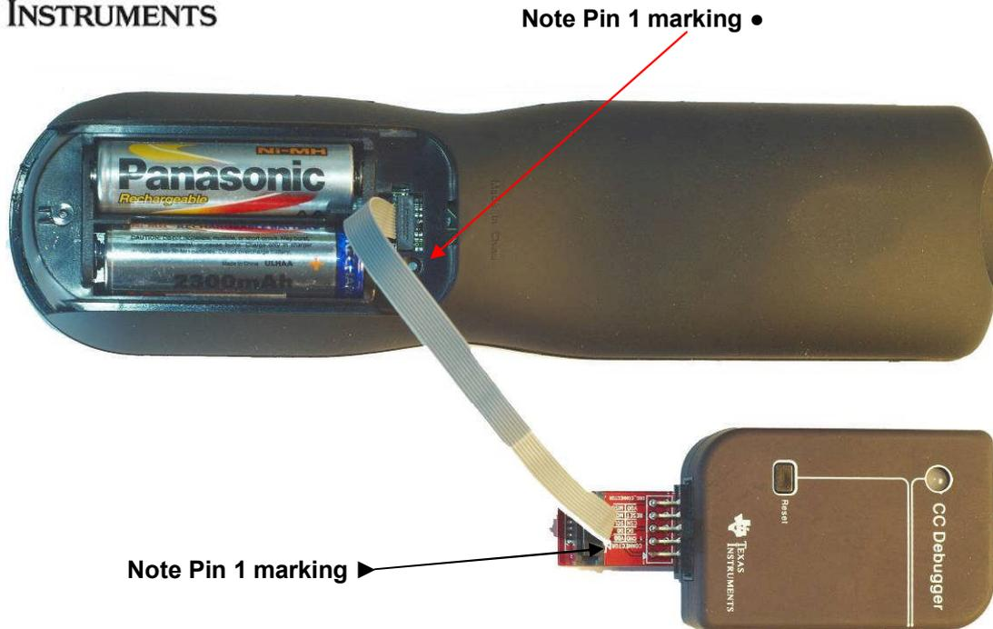
**Figure 9: Connecting the remote control to the CC Debugger**
