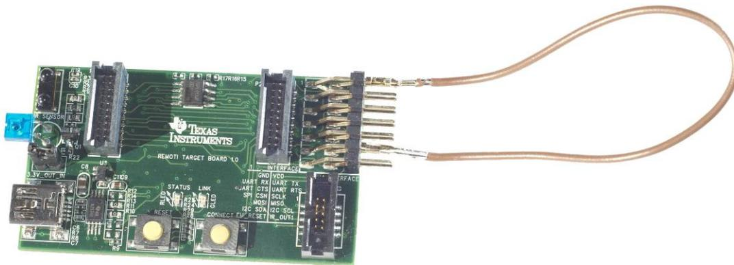
**Figure 16: Short pin 1(GND) and pin11 (SDA)**
